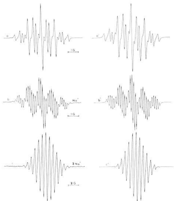
Figure 2. ESR spectra for reduced syn -BiP in THF: (a) experimental and (a') simulation; (b) in the presence of 1 equiv of \text{Na}^+ and (b') simulated; (c) with 2 equiv of \text{Na}^+ and (c') simulated.
